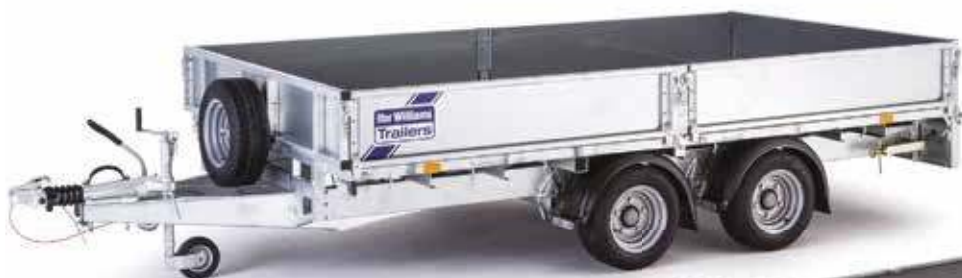
LM126 with optional dropsides, tailboard and headboard.
